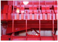
DFCS disengaged for maximum flow through the flywheel.
