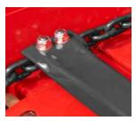
The conveyor slats are designed for quick and easy individual replacement.
