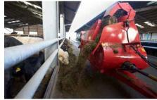
The hydraulically driven swivel chute operates in 4 stages which optimises the blowing distance when bedding.
