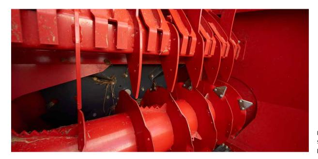
Improved aggressive shredder rotor for quick processing of material.
