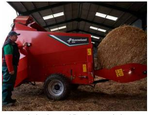
Operating both tailgate and floor chain in safe distance from the moving parts, by using the remote control placed on the side of chamber.
