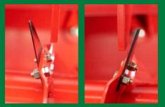
A Kverneland patented system the knives pass the fixed comb on alternative sides for a more even cut.
