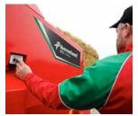
Operating both tailgate as well as floor chain in a safe distance from the moving parts by using the remote control placed on the side of the 853 Pro.
